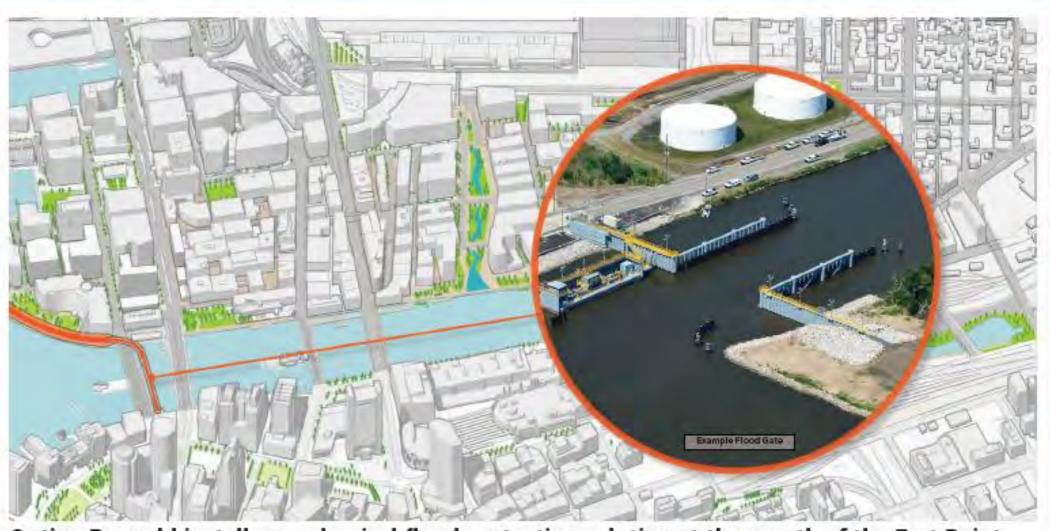
Option B would install a mechanical flood protection solution at the mouth of the Fort Point Channel
